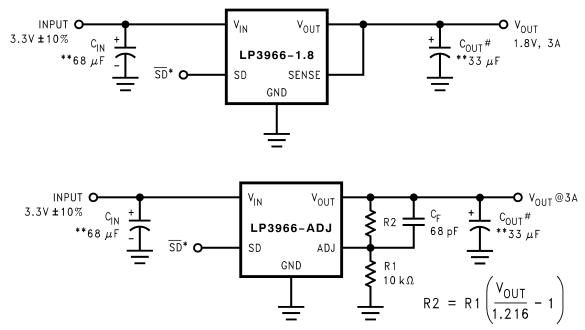
\*SD and ERROR pins must be pulled high through a  $10k\Omega$  pull-up resistor. Connect the ERROR pin to ground if this function is not used. See Application Hints for more information.
