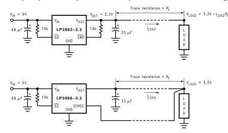
Figure 22. Improving remote load regulation using LP3966
