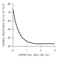
Figure 23. θ<sub>JA</sub> vs Copper (1 Ounce) Area for DDPAK/TO-263 package
