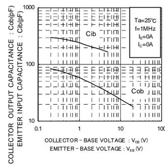
Fig.6 Emitter Input Capacitance vs. Emitter-Base Voltage
