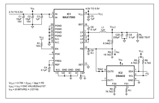
Figure 1. Using the DS4432 I<sup>2</sup>C-controlled digital-to-analog converter (DAC) to inject current into the feedback node of the MAX17083 step-down regulator enables I<sup>2</sup>C control of the regulator's output voltage.
