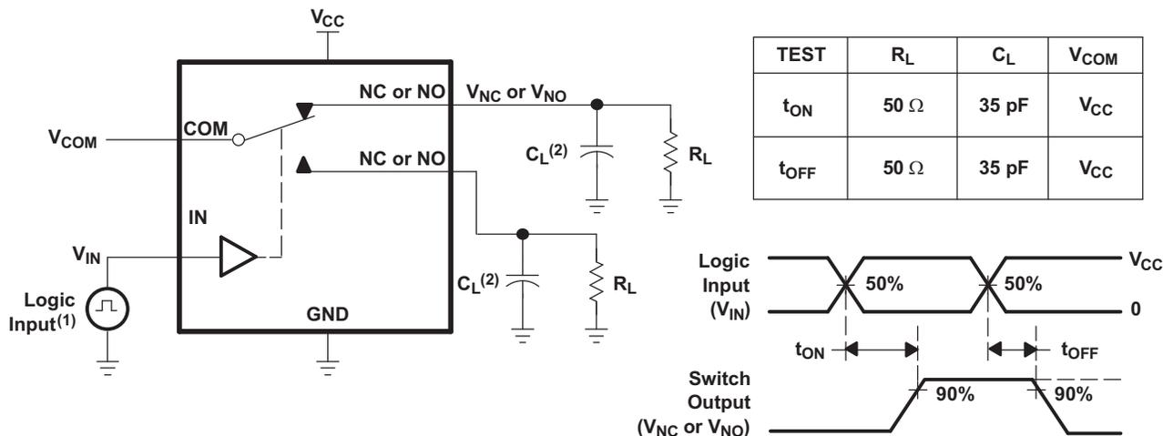
(1) All input pulses are supplied by generators having the following characteristics:
