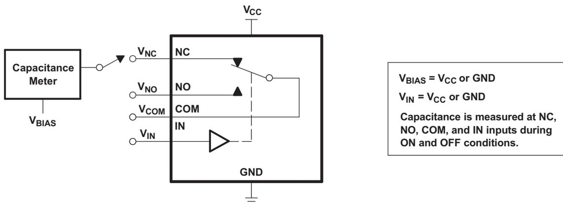
$C_I, C_{COM(ON)}, C_{NC(OFF)}, C_{NO(OFF)}, C_{NC(ON)}, C_{NO(ON)}$
