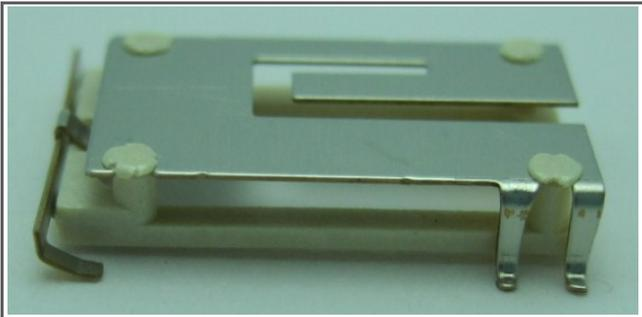
Ethertronics' Prestta series of Isolated Magnetic Dipole™ (IMD) stamped metal antennas include an embedded Bluetooth design that delivers on the key needs of today's wireless product designers: **miniaturized design, superior signal sensitivity and high isolation properties** that virtually **eliminate de-tuning**. Together, these features provide compelling advantages for IMD-enabled cell phones, handsets headphones, laptops and other wireless devices that utilize Bluetooth technology.
