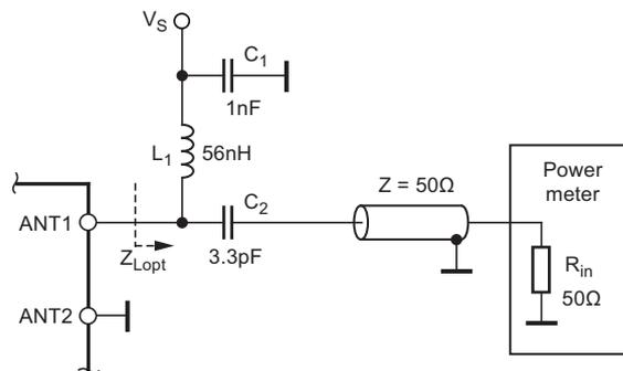
Note: For 345MHz  $C_2$  has to be changed to 2.7pF
