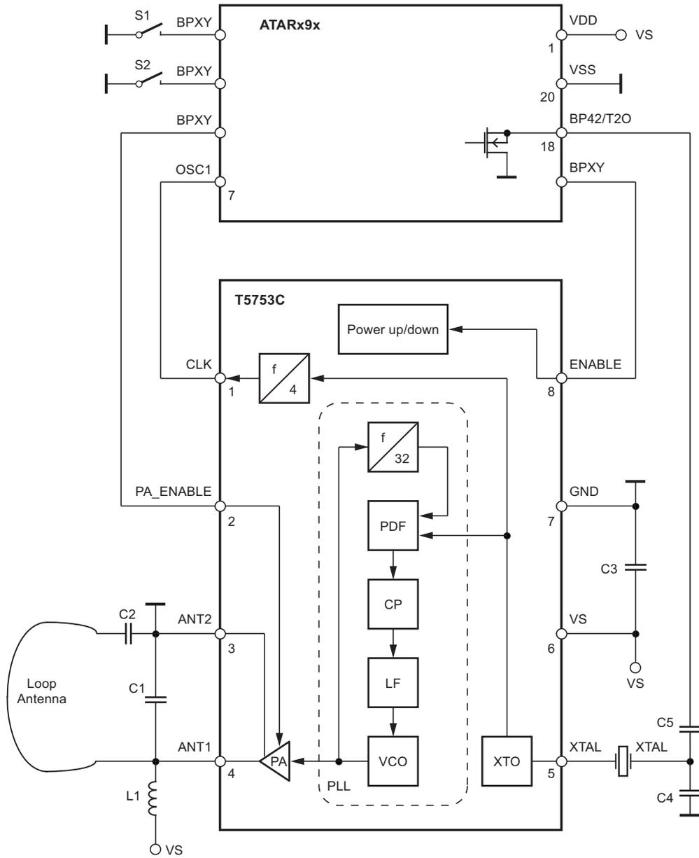
Figure 4-5. ESD Protection Circuit
