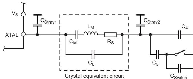
Using  $C_4 = 8.2\text{pF} \pm 5\%$ ,  $C_5 = 10\text{pF} \pm 5\%$ , a switch port with  $C_{Switch} = 3\text{pF} \pm 10\%$ , stray capacitances on each side of the crystal of  $C_{Stray1} = C_{Stray2} = 1\text{pF} \pm 10\%$ , a parallel capacitance of the crystal of  $C_0 = 3.2\text{pF} \pm 10\%$  and a crystal with  $C_M = 13\text{fF} \pm 10\%$ , an FSK deviation of  $\pm 21.5\text{kHz}$  typical with worst case tolerances of  $\pm 16.25\text{kHz}$  to  $\pm 28.01\text{kHz}$  results.
