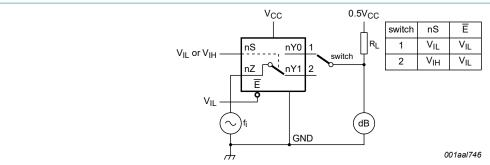
Adjust f<sub>i</sub> voltage to obtain 0 dBm level at output. Increase f<sub>i</sub> frequency until dB meter reads -3 dB.
