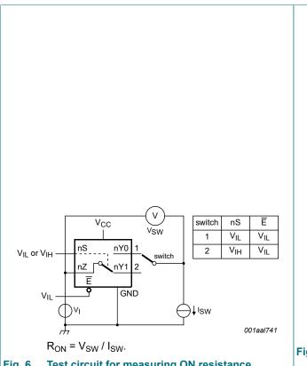
Test circuit for measuring ON resistance
