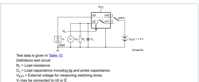
Fig. 16. Test circuit for measuring switching times
