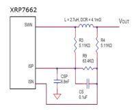
Fig. 20: Over Current Detection Circuit for  $I_{MAX}$ >60mV/DCR
