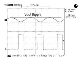
Fig. 4: Output Ripple, No Load
