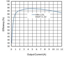
Fig. 15: Efficiency versus  $I_{\text{OUT}}$ ,  $V_{\text{IN}}$ =12V,  $V_{\text{OUT}}$ =1.2
