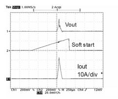
Fig. 11: Output Short Circuit
