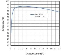
Fig. 14: Efficiency versus  $I_{\text{OUT}}$ ,  $V_{\text{IN}}$ =5.5V,  $V_{\text{OUT}}$ =1.2
