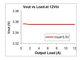
Fig. 13: Vout versus Load Current, VIN=12V
