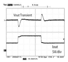
Fig. 9: Load Step Response, I<sub>OUT</sub>=6A-12A
