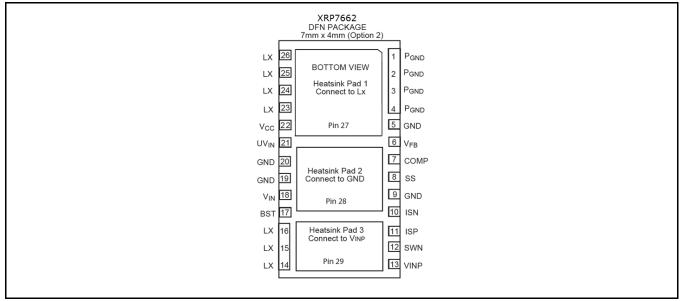
Fig. 3: XRP7662 Pin Assignment
