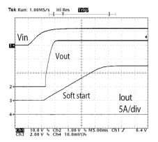
Fig. 6: Startup Response, No Load
