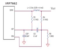
Fig. 21: Over Current Detection Circuit for I<sub>MAX</sub><(60mV/DCR)
