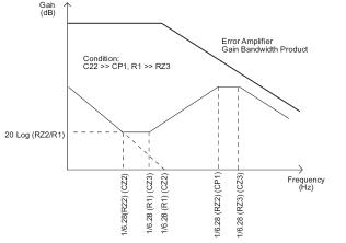
Fig. 23: Bode Plot of Type III Error Amplifier Compensation
