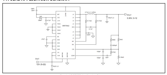
Fig. 1: XRP7662 Application Diagram
