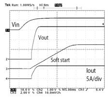
Fig. 7: Startup Response, IOUT=6A
