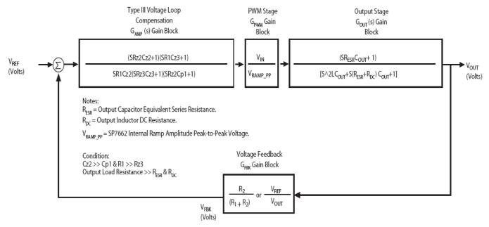
Fig. 22: XRP7662 Voltage Mode Control Loop with Loop Dynamic
