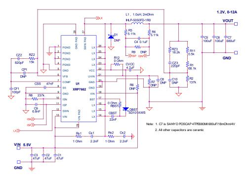
Fig. 16:  $5.5V_{IN}$  test circuit
