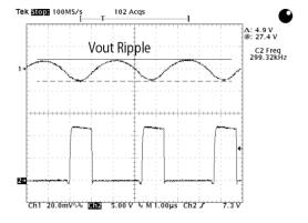
Fig. 5: Output Ripple, I<sub>OUT</sub>=12A
