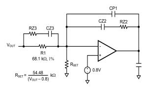
Fig. 24: Type III Error Amplifier Compensation Circuit
