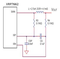
Fig. 19: Over Current Detection Circuit
