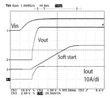
Fig. 8: Startup Response, I<sub>OUT</sub>=12A
