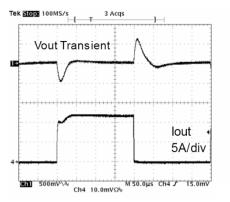
Fig. 10: Load Step Response,  $I_{OUT}$ =0A-12A
