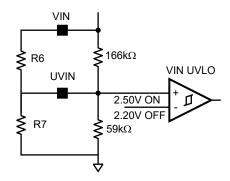
Fig. 18: Internal and External Bias of UVIN
