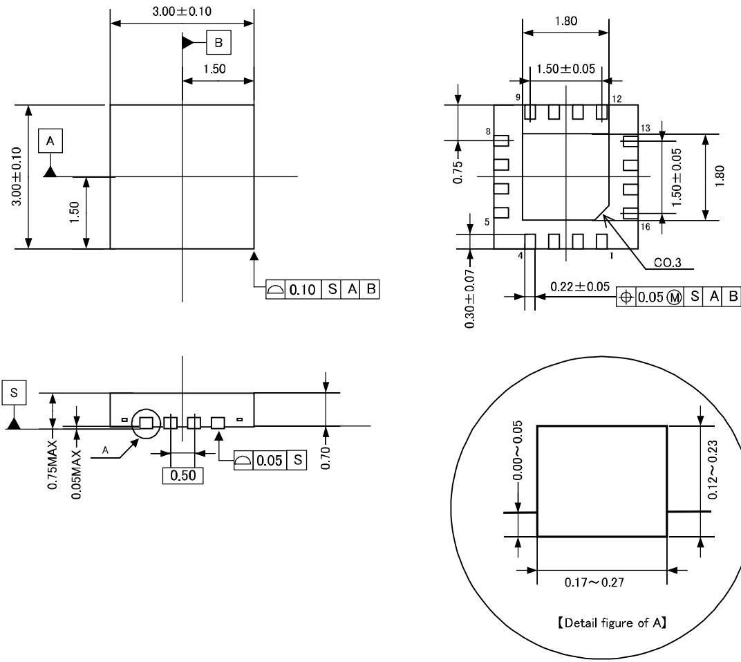
Note The exposed pad at the center of the back of the package must be connected to VSS or opened.
